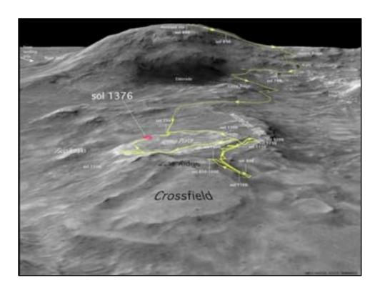
Here's a map based on a photograph taken from Mars orbit. It shows how Spirit traveled from its landing site in Gusev crater about 100 meters up and over the Columbia Hills and down onto a kind of plateau called Home Plate.
