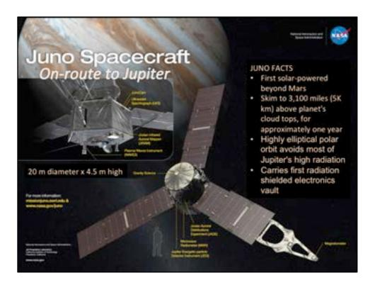
Another spacecraft called Juno is on its way to Jupiter. It's the first solar powered spacecraft to operate so far from the sun, so It's quite large, about 60 feet across. With a polar orbit and radiation shielding to protect the electronics, Juno will fly within about 5000 km of the surface clouds in a one year mission.
