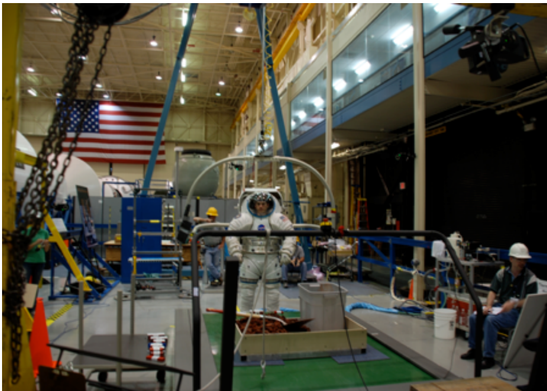
Figure 1. Astronaut in pressurized suit suspended by Partial Gravity Simulator (POGO) at Johnson Space Center (2007)
