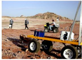
Image left: EVA configuration with Tropos relay to hab (on trailer) and John Ossenfort, from NASA Ames, operating the ATV that simulates Thibodeaux (display mounted up front indicates commands received by Thibodeaux from the agent system). Geologist Abby Semple told Thibodeaux to follow her; Ossenfort carries out necessary movements indicated by the display. Image courtesy: NASA.
