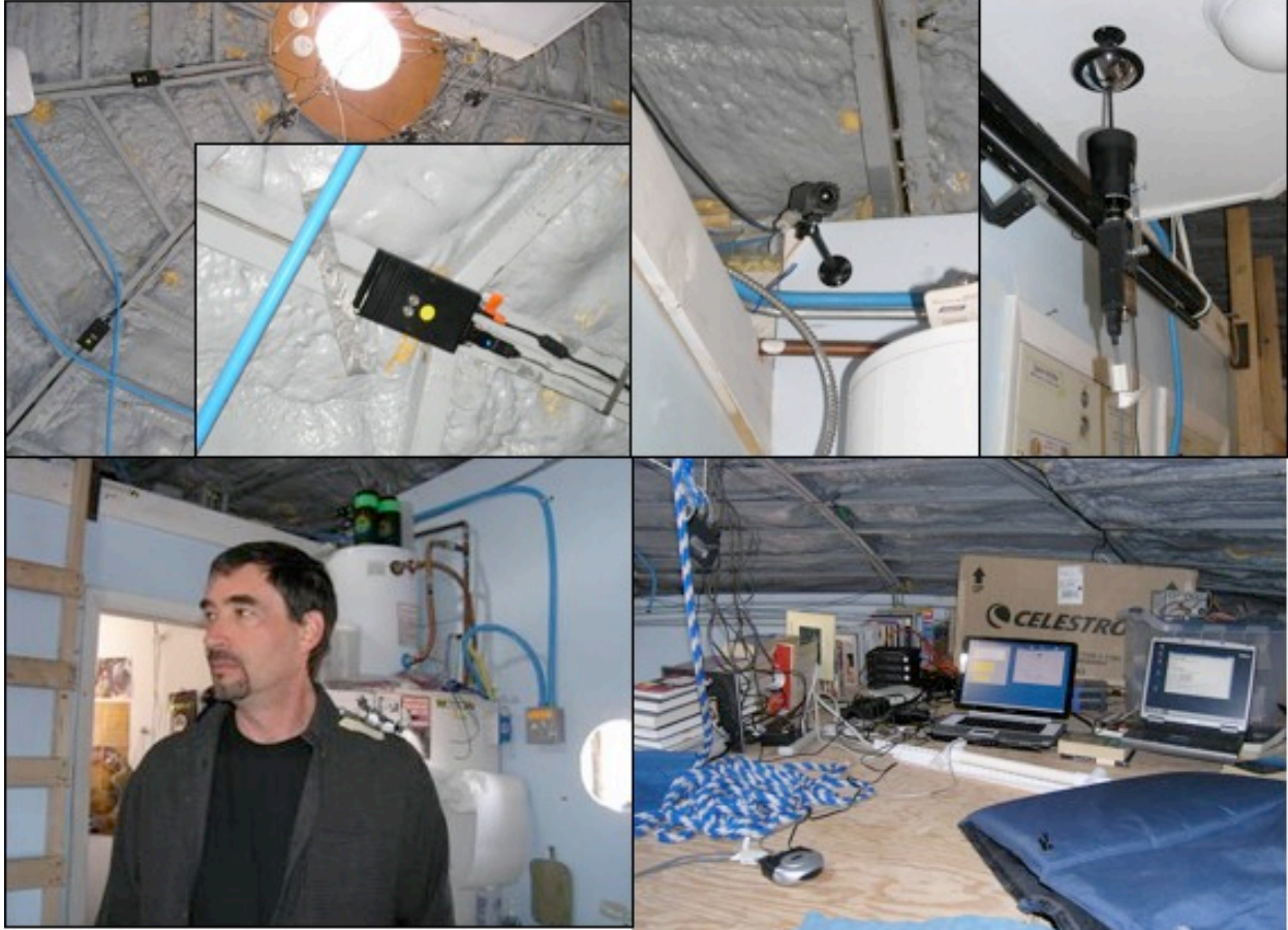
Figure 7. Implementation of Crew Activity Analyzer (from bottom left): “Cricket” wireless transmitters are placed on crew member’s shoulders or worn on a hat (not shown: each crew member wears a wireless microphone); detectors are arrayed on ceiling of upper deck; one camera is above galley and 180 degree fisheye hangs above center stateroom door; computers in loft record and synchronize audio, video, and crew locations. (All photos by Clancey, except lower left by Jim Murray, Foster-Miller, Inc.)
