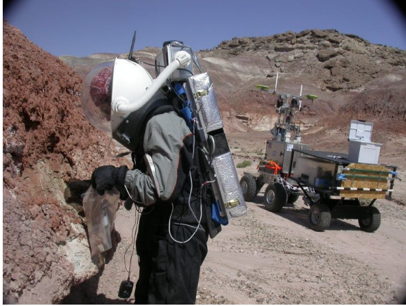
Figure 2. An Astronaut-Scientist collects a sample during a simulated EVA using MAA at the MDRS. Cameras on the EVA Robotic Assistant (ERA) can automatically track the Astronauts and relay the video back to the Habitat. A science trailer, used to carry field equipment and samples, is attached to the ERA. Photo by W. J. Clancey (NASA).
