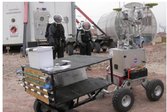
Figure 1. Two astronaut-geologists and the ERA with science trailer prepare to leave the MDRS during a simulated EVA in the Utah desert. Image courtesy of NASA.
