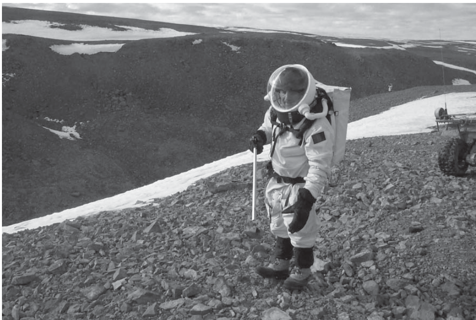
Fig. 5 Rocks can be collected from the ground without bending down in cumbersome suits by using a grappling tool.
