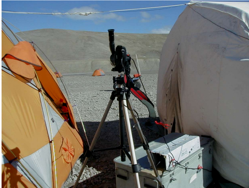
Figure 3: Example placement of camera for time-lapse video, recording entry and exit from dome and work tents, plus the central staging area used for traverse preparation.
